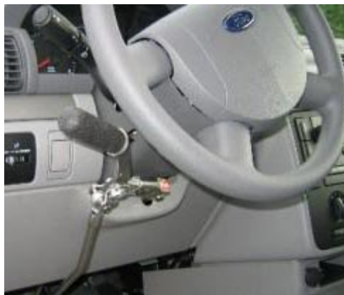
MPS Monarch Mark 1-A Hand Controls at Sacramento Van Conversions
